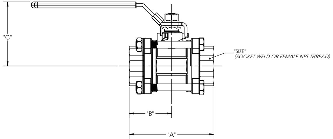
1. DIMENSIONS ARE APPROXIMATE AND MAY VARY FROM VALVE TO VALVE. REFERENCE VALEX SPECIFICATION SP-9236 FOR OVERALL LENGTH TOLERANCES.
